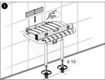
Determine the user height of the seat and measure this height against the wall. Adjust the feet to make finer adjustment. Remove the bracket cover.
