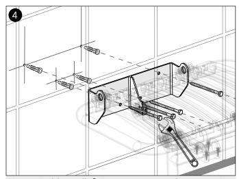
Use suitable wall fixings to secure the mounting bracket to the wall. Do not use countersunk screws as this can reduce the strength of the seat and will invalidate any warranty or weight capacity stated.
