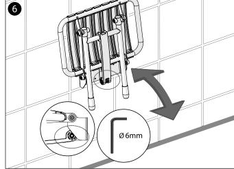
To adjust the rate the seat lowers, tighten or loosen the linkage bolt under the seat with a 6mm Allen key.
