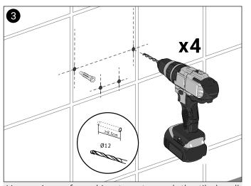
Use a piece of masking tape to mark the tiled wall and to protect the tile from splintering. Drill the holes with a suitable wall / tile drill piece. Fixings not supplied.
