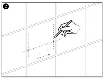
Mark the position of the mounting bracket holes on the wall ensuring the seat is level. Check for any obstacles or pipework before any drilling or fixing.
