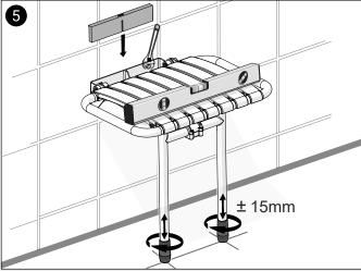
Do not over-tighten fixings. Check the seat operation, levels and leg positioning when it is raised and lowered. Replace the bracket cover.
